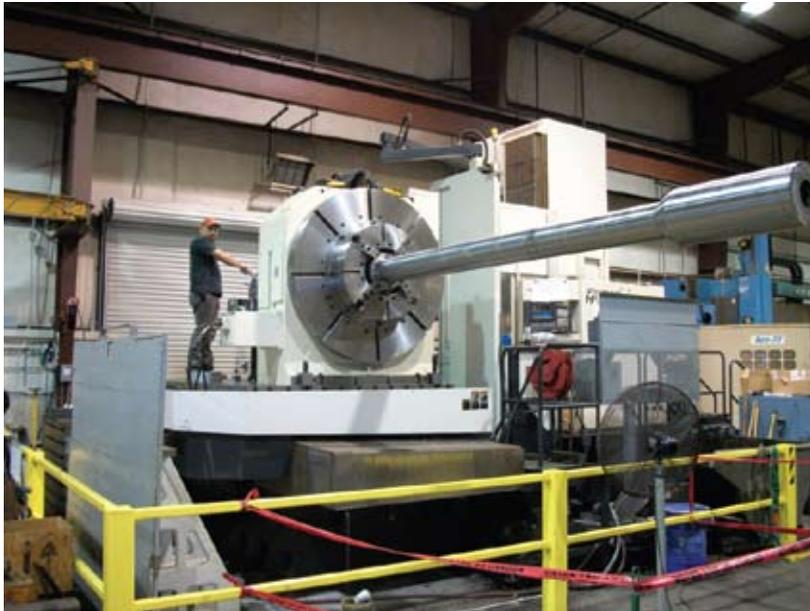
***RTI Energy Systems (Spring, TX) a subsidiary of RTI International Metals, was able to expand its machining capabilities by acquiring a Tsudakoma RNCV1501 1.5-m NC rotary table from Koma Precision Inc. to handle deepwater component that was 20' (6-m) long and weighed 6000 lb (2721 kg).***
