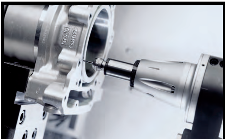
Automatic insertion of angle head through machines tool changer
