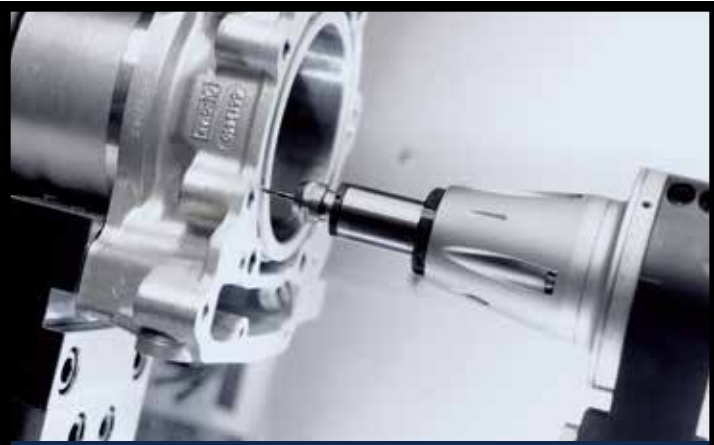
Automatic insertion of angle head through machines tool changer
