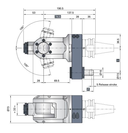
Direction of rotation opposite to machine spindle
