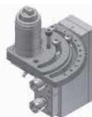
TSB596200 2 spindle drilling/milling unit RATIO 1 : 1 RPM(MAX) 6000 TOOL CLAMPING ER16M ANGLE ADJUSTMENT 0~90° TSUGAMI ITEM NO. 3282-Y921
