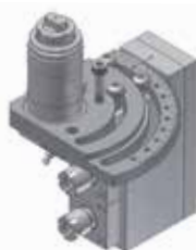
TSB496200 2 spindle drilling/milling unit RATIO 1 : 1 RPM(MAX) 6000 TOOL CLAMPING ER16M ANGLE ADJUSTMENT 0~90°
